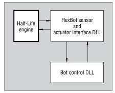
Figure 1. The FlexBot architecture design.
