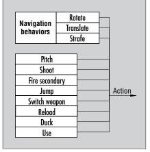
Figure 4. Combining outputs from individual behavior sets to form a single action vector that is sent to the Half-Life engine.
