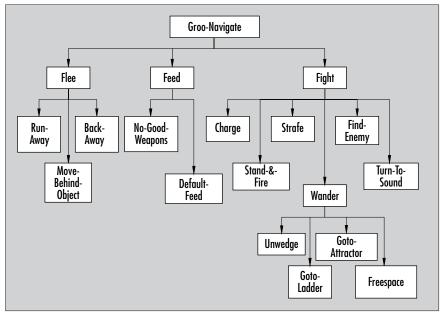
Figure 2. Groo navigation behaviors. On every program cycle, the navigation behavior with the highest activation level wins and gets to dictate the Groo bot's current rotate, translate, and strafe values.
